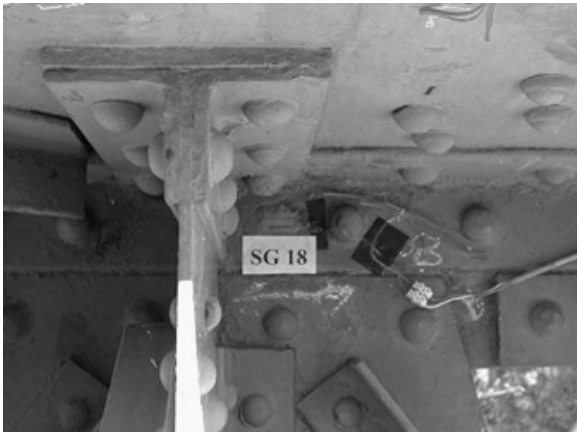
Fig. 9. Strain gage placed at location S_{18} .
