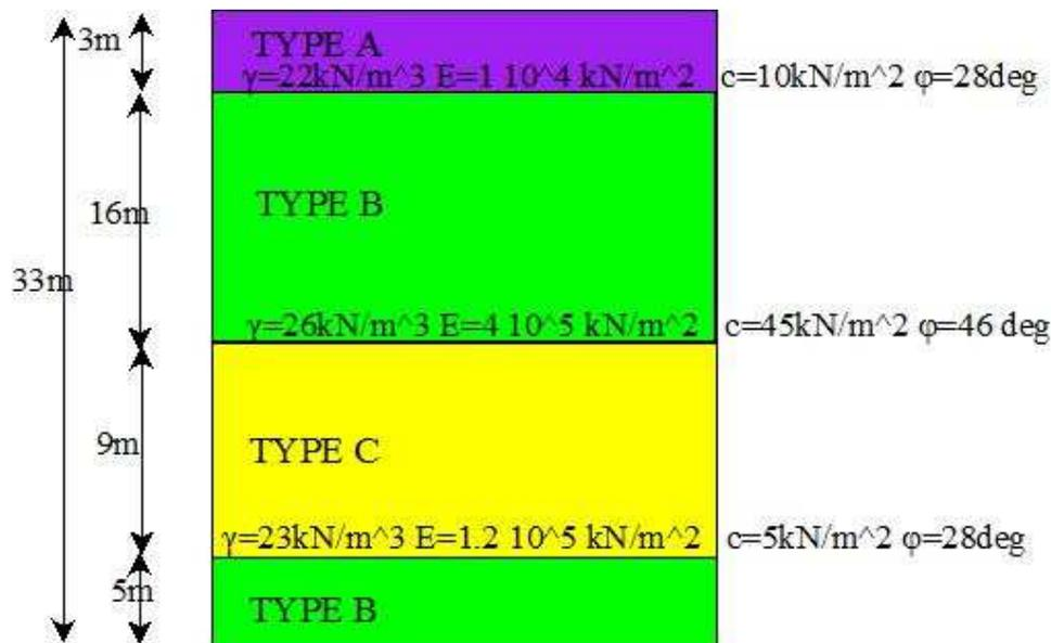
*Figure 1 – The soil profile and characteristics*
