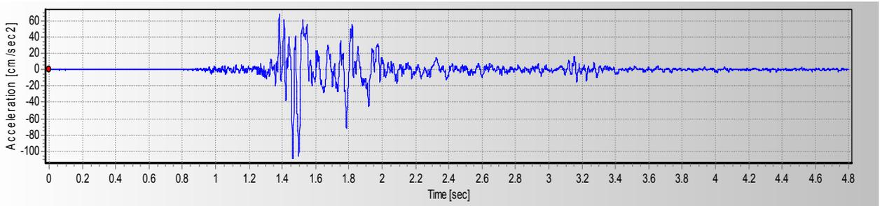
Figure 4 – Syntagma (Athens) 1999 earthquake record on the bedrock,
