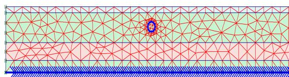
Figure 2b – The finite element mesh of Plaxis model
