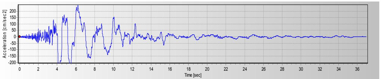
Figure 5 – Kobe (Japan) 1995 earthquake record on the bedrock,
